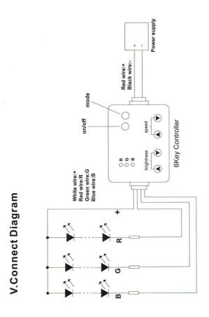
IR 6key Controller is specially designed for controlling LED multicolor changing patterns. Its slim and delicate shape enables a no-sweat installation. The design flexibility on LED fittings will be enhanced enormously. The remote controlling system is to make your home decoration possible with industrial products.
